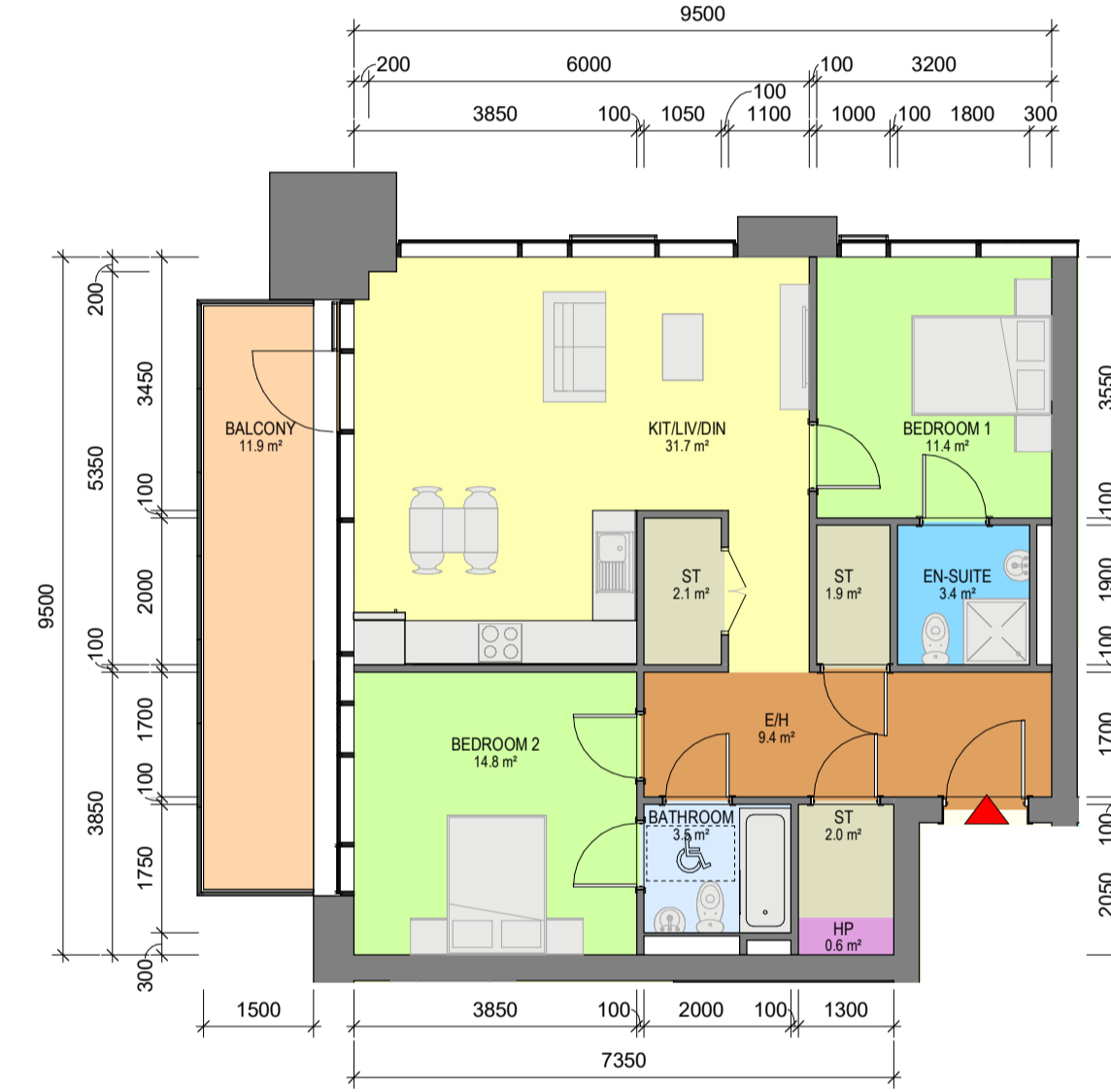
8 Apartment Type 2H 1 : 100 - 2 BED, 4 PERSON APARTMENT - NET INTERNAL AREA (NIA) Areas shown in plan - GROSS INTERNAL AREA (GIA) : 85.44sqm
