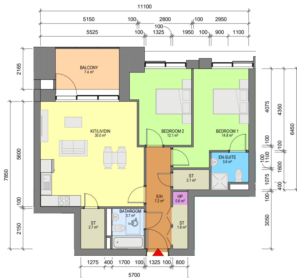
10 Apartment Type 2J 1 : 100 - 2 BED, 4 PERSON APARTMENT - NET INTERNAL AREA (NIA) Areas shown in plan - GROSS INTERNAL AREA (GIA) : 83.01sqm
