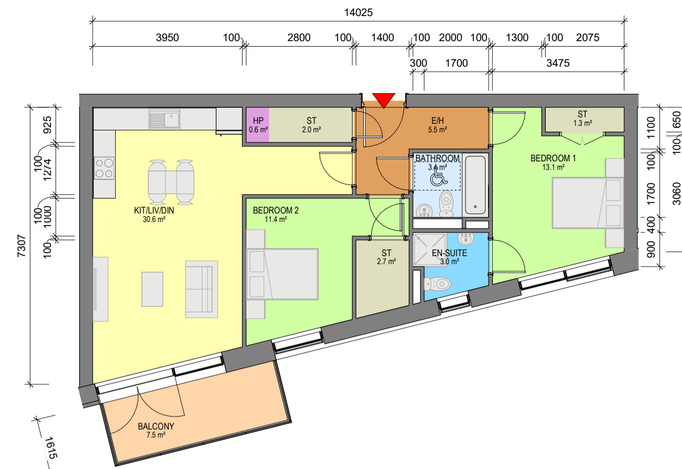
4 Apartment Type 2D 1 : 100 - 2 BED, 4 PERSON APARTMENT - NET INTERNAL AREA (NIA) Areas shown in plan - GROSS INTERNAL AREA (GIA) : 77.96sqm
