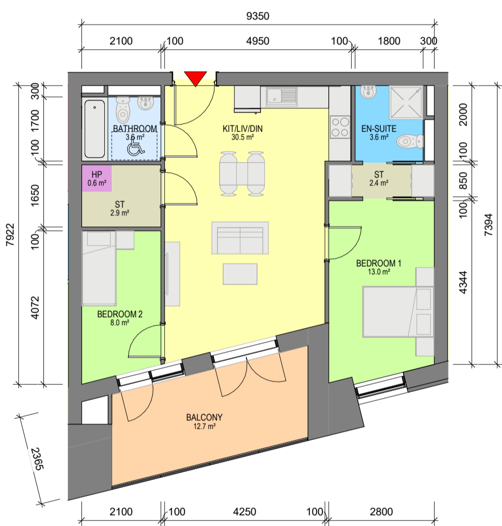
5 Apartment Type 2E 1 : 100 - 2 BED, 3 PERSON APARTMENT - NET INTERNAL AREA (NIA) Areas shown in plan - GROSS INTERNAL AREA (GIA) : 68.11sqm
