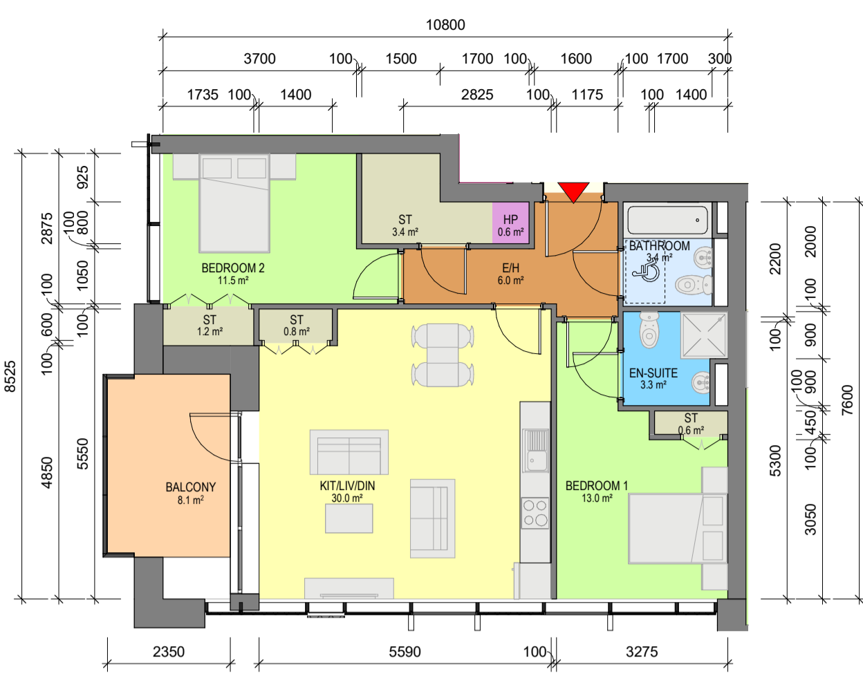
2 Apartment Type 2B 1 : 100 - 2 BED, 4 PERSON APARTMENT - NET INTERNAL AREA (NIA) Areas shown in plan - GROSS INTERNAL AREA (GIA) : 78.09sqm
