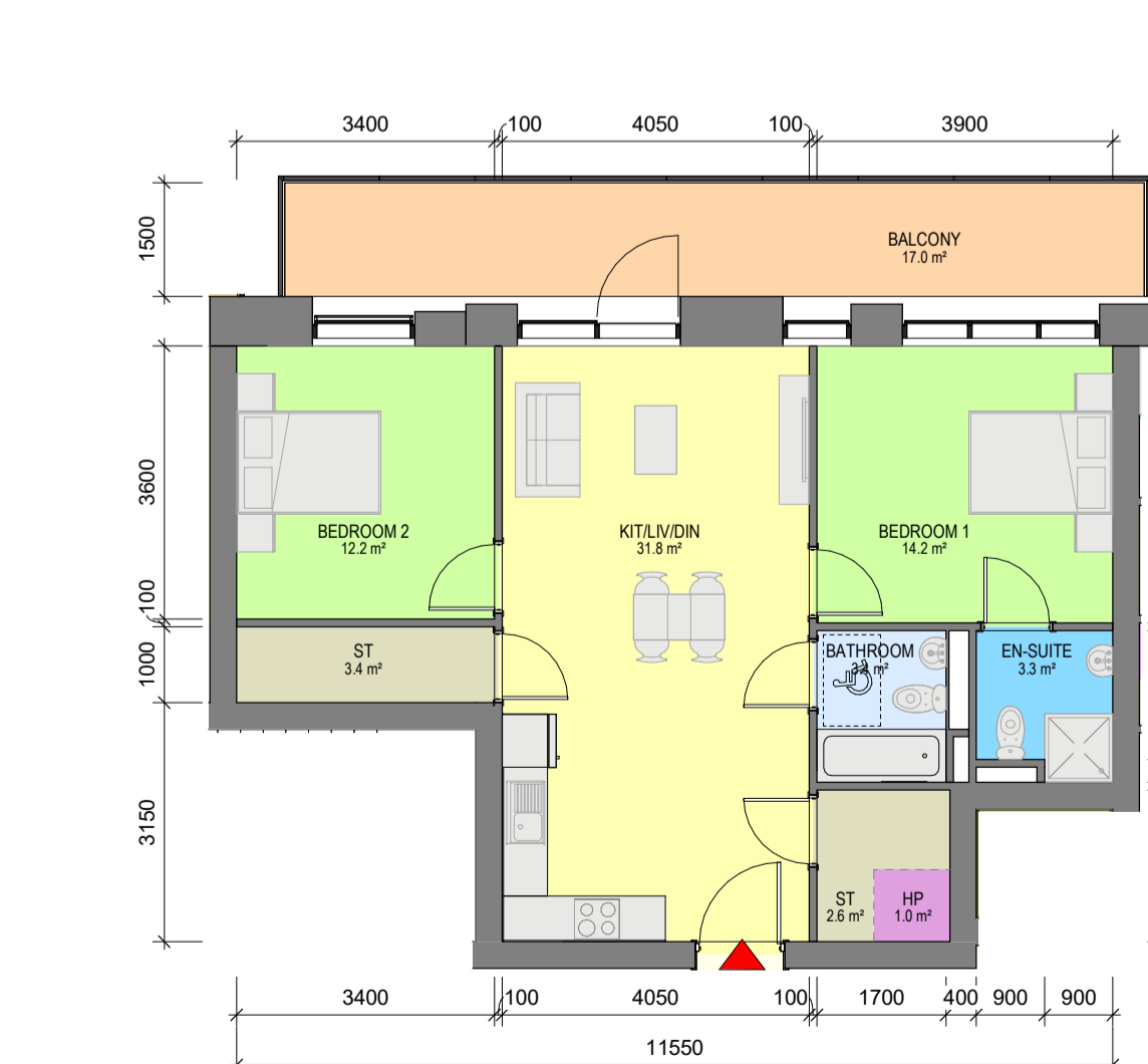
12 Apartment Type 2L 1 : 100 - 2 BED, 4 PERSON APARTMENT - NET INTERNAL AREA (NIA) Areas shown in plan - GROSS INTERNAL AREA (GIA) : 75.13sqm
