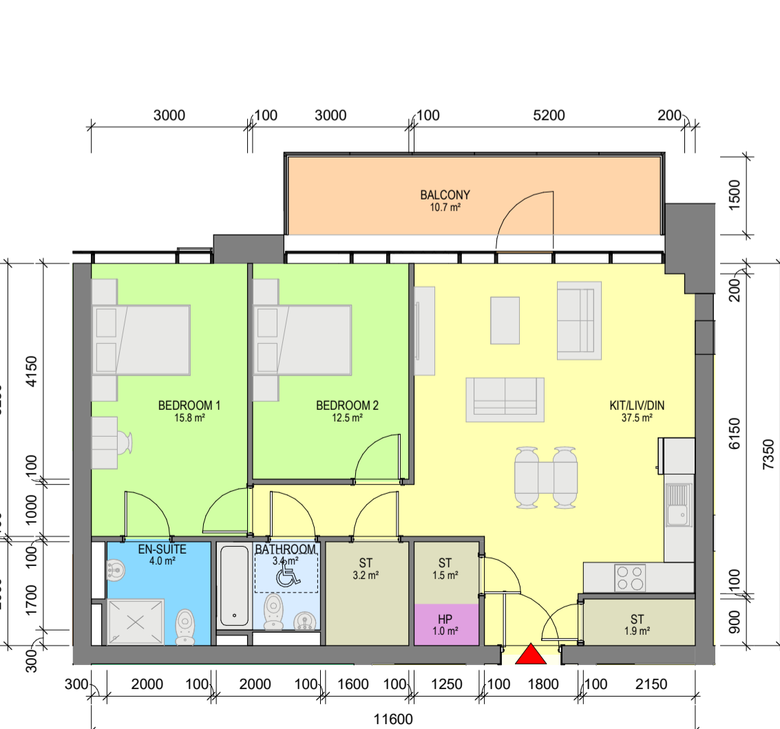
9 Apartment Type 2I 1 : 100 - 2 BED, 4 PERSON APARTMENT - NET INTERNAL AREA (NIA) Areas shown in plan - GROSS INTERNAL AREA (GIA) : 85.07sqm
