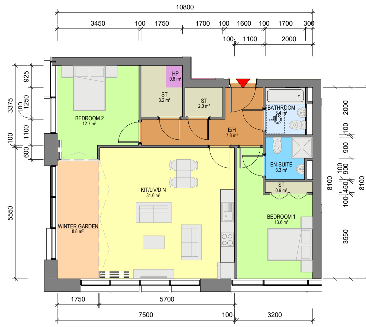
3 Apartment Type 2C 1 : 100 - 2 BED, 4 PERSON APARTMENT - NET INTERNAL AREA (NIA) Areas shown in plan - GROSS INTERNAL AREA (GIA) : 83.29sqm
