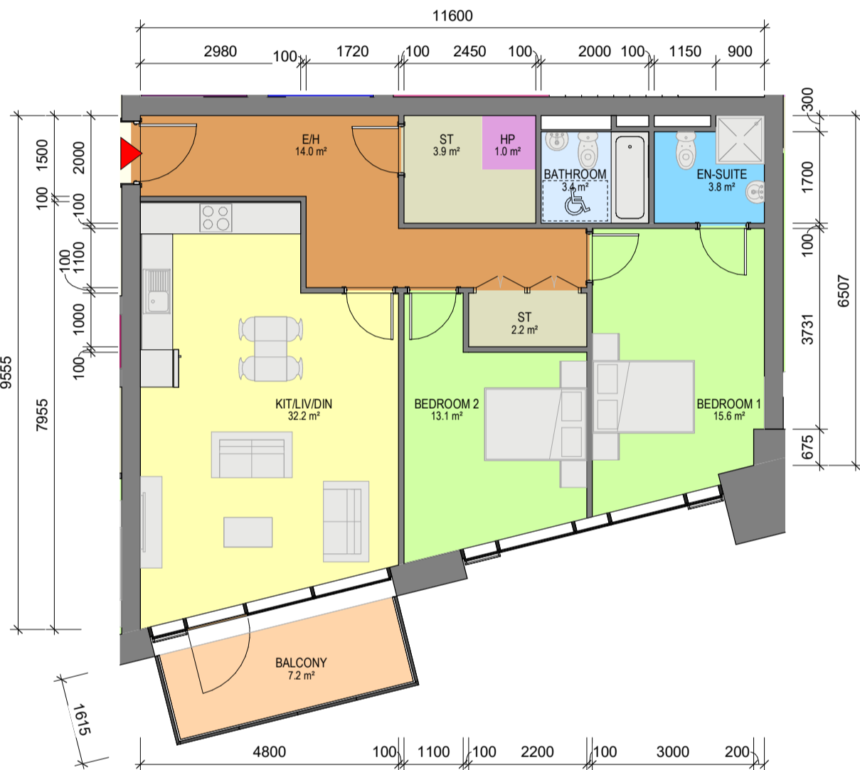
6 Apartment Type 2F 1 : 100 - 2 BED, 4 PERSON APARTMENT - NET INTERNAL AREA (NIA) Areas shown in plan - GROSS INTERNAL AREA (GIA) : 93.76sqm
