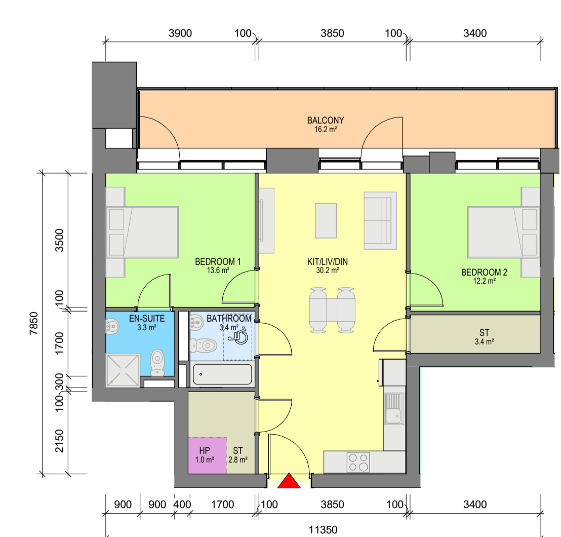
11 Apartment Type 2K 1 : 100 - 2 BED, 4 PERSON APARTMENT - NET INTERNAL AREA (NIA) Areas shown in plan - GROSS INTERNAL AREA (GIA) : 73.24sqm
